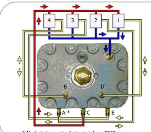
Solenoid valves are numbered in unloading sequence.
