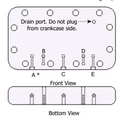
\* No hole is required at point A on 5F40 compressors.
