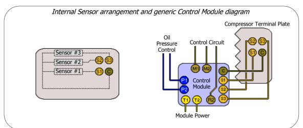
Use and ohmmeter with no more than 3 volt batteries. Check resistance from common terminal to each of the other sensor terminals. The module trip point is 100 ohms. Each sensor should read between 65 and 105 ohms depending on their temperature. If an internal sensor should fail it may be bypassed using a 75 - 80 ohm 1/4 watt resistor. This will reduce the effectiveness of the electronic motor protection system but will allow the compressor to operate.
